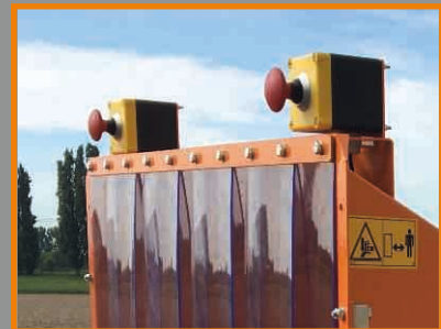
Emergency buttons on funnel or top cover.
