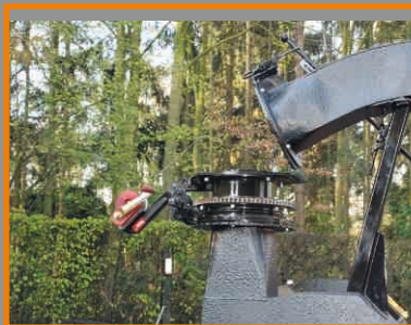
Manual winch to lower the discharge chute.
