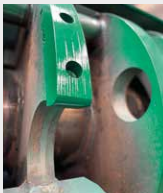
Chamfering on the rotor discs
