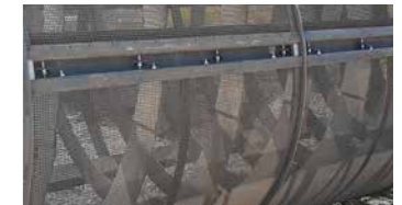
Screening trommel with wire segments
