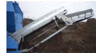
Stone separation belt for rolling material
