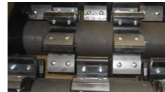
Wear plates on polyurethane screening stars
