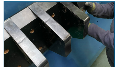
Single bolted comb elements
