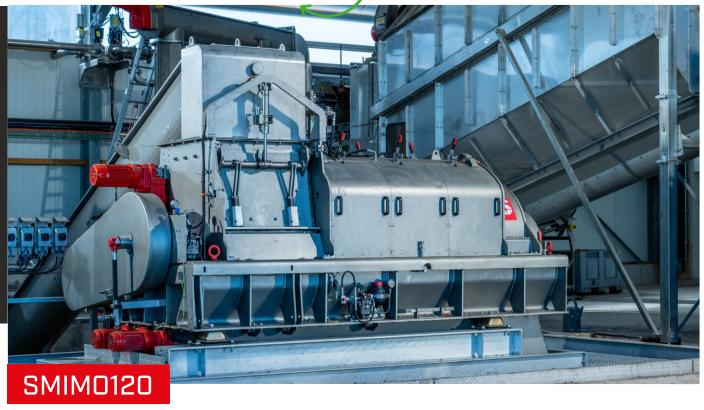
The SMIMO120 is perfect for separating organic products (supermarket returns and/or residual streams from food production) from its packaging with the organic part being finely ground. The SMIMO120 is a machine that can process large quantities up to 35 m<sup>3</sup> per hour. The machine is fitted for seperating both dry and moist product.
