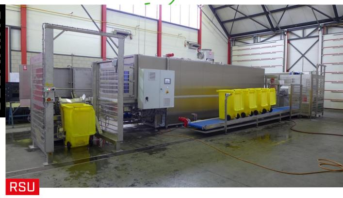
With a cleaning unit, multiple kinds of containers can be washed and cleaned. The insulated walls make sure that the washing unit operates very energy saving. Besides, the unit has a quite low water consumption. The cleaning unit can be equipped with an automatic feeding tipper and discharge system.
