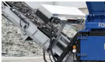
Hydraulically adjustable magnet (also F 38)
