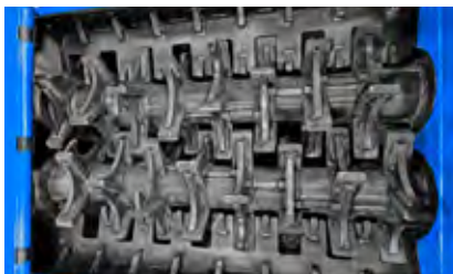
Individually adjustable shaft speeds (also F 25)
