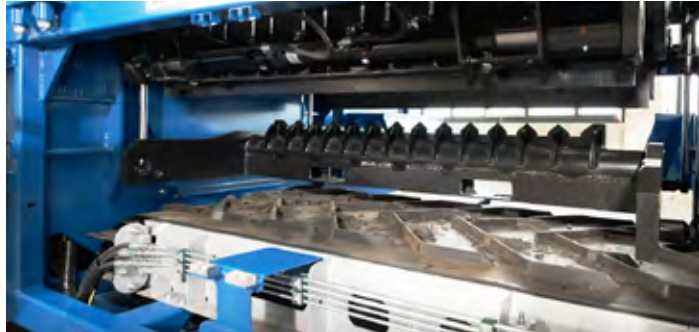
Definition of the final grain size via various after breaker bars and screen baskets
