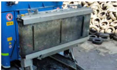
Powerful neodymium magnet with discharge on both sides (also Z 60)
