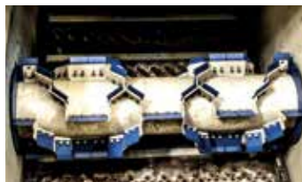
Rotor with swivel unit
