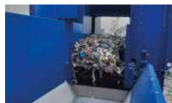
Steel plate bale conveyor
