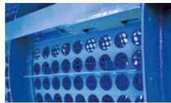
Entanglement protection with flat bars
