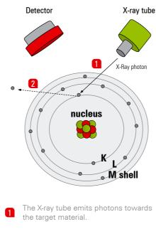
2 The electron is ejected out of the atomic shell, which creates a free spot.
