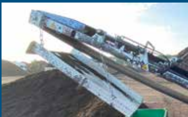
Magnetic rollers - to separate iron on discharge belt
