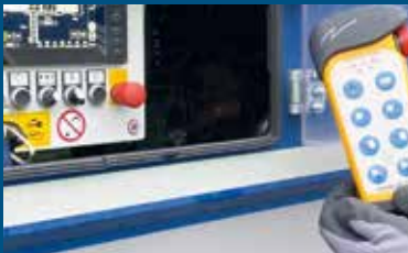
Radio remote control - to control from the wheel loader
