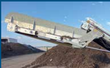
Stone belt - to separate stones and heavy impurities
