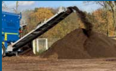
Long belts - for bigger ejection heights
