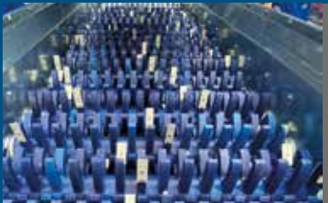
SCREENFIX - star screening deck
