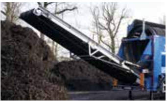
Extended coarse grain belt, discharge height of up to 3,800 mm
