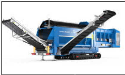
TERRA SELECT T 60 with track drive
